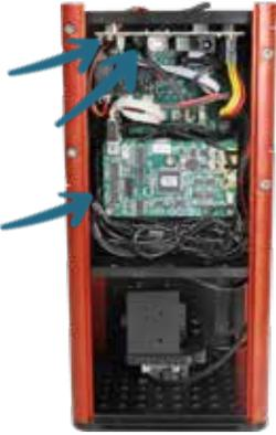
unscrew three bolts that hold miniRaman spectrometer
