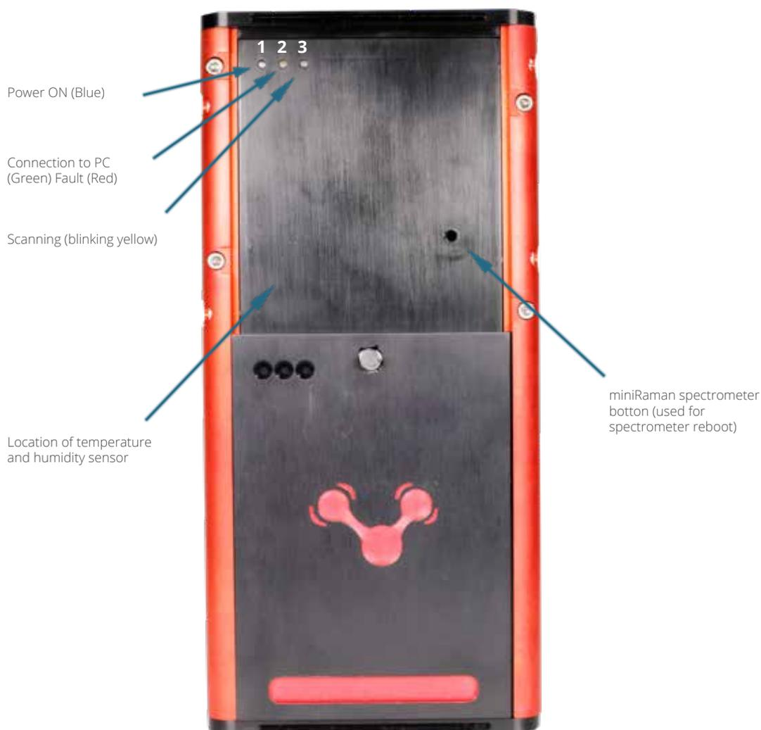
Figure 8. LED indicators of miniRaman microscope.
