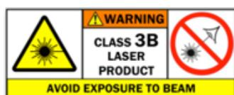
This warning symbol indicates the existence of laser radiation. Class 3B lasers *are hazardous for eye exposure*. They can heat skin and materials but are not considered a burn hazard. For visible-light lasers, Class 3B lasers' output power is between 5 and 499 milliwatts. Class 3B lasers are *normally hazardous under direct beam viewing conditions*, but are normally safe when viewing diffuse reflections.
