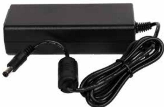
Please remove power adaptor (Figure 4) and connect it to the right connector on the rear panel of the miniRaman microscope (Figure 5). Then connect USB cable to the left connector on the rear panel and connect it to PC from the other side.
