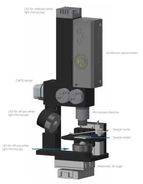
Figure 7. Opto-mechanical design of the miniRaman microscope.
