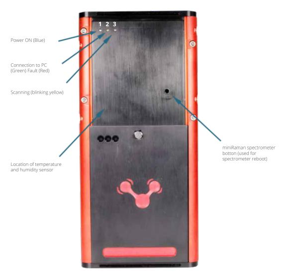
Figure 8. LED indicators of miniRaman microscope.
