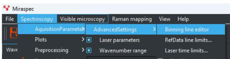
**Figure 14.** miniRaman spectroscopy settings; advanced settings menu.
