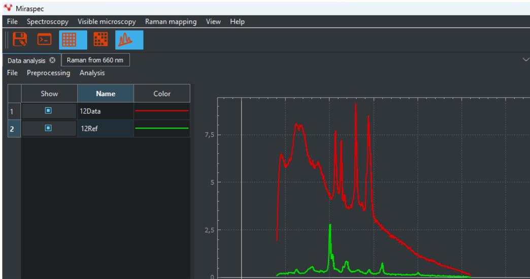
**Figure 26.** Raw spectra (red) and reference spectrum (green). “Show” tab enables to visualize desired spectra.
