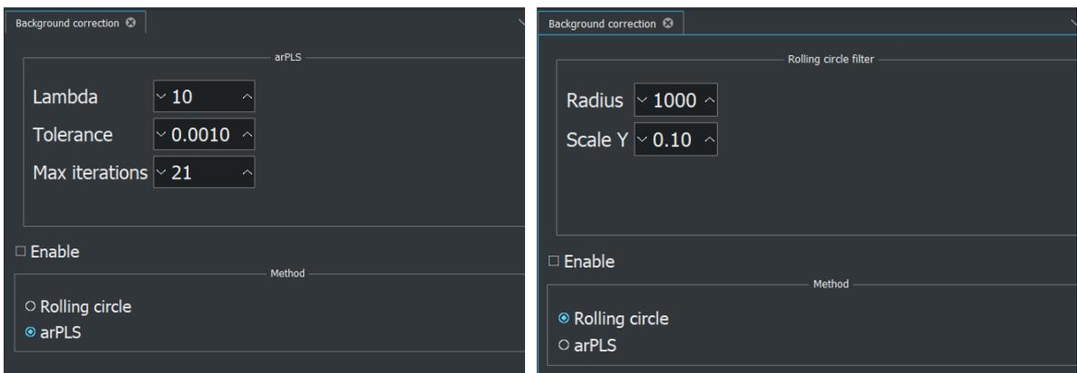
**Figure 21.** Background correction methods. Left panel – arPLS algorithm, right panel – Rolling circle.
