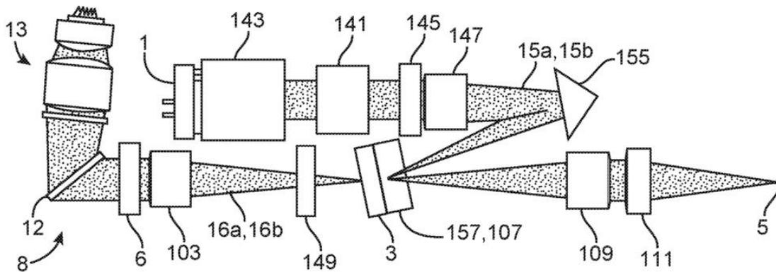
**Figure 4.** Optical schema of MiniRaman spectrometer. See details for patent # US20210072158 here: <https://patentscope.wipo.int/search/en/detail.jsf?docId=WO2019145005> .
