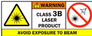
This warning symbol indicates the existence of laser radiation. Class 3B lasers are hazardous for eye exposure. They can heat skin and materials but are not considered a burn hazard. For visible-light lasers, Class 3B lasers' output power is between 5 and 499 milliwatts. Class 3B lasers are normally hazardous under direct beam viewing conditions, but are normally safe when viewing diffuse reflections.
