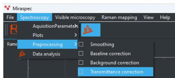
**Figure 19.** Different options for spectra preprocessing.
