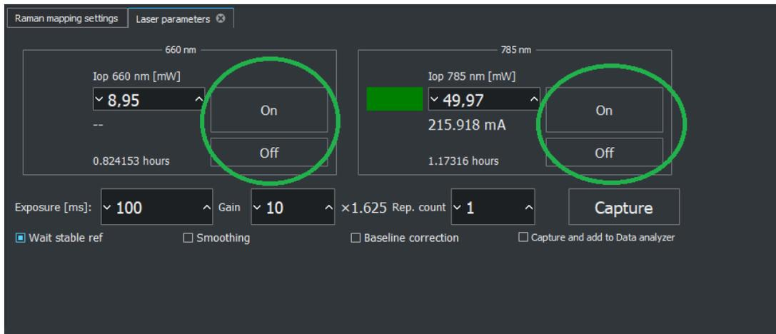
**Figure 9.** Switching on/off laser
