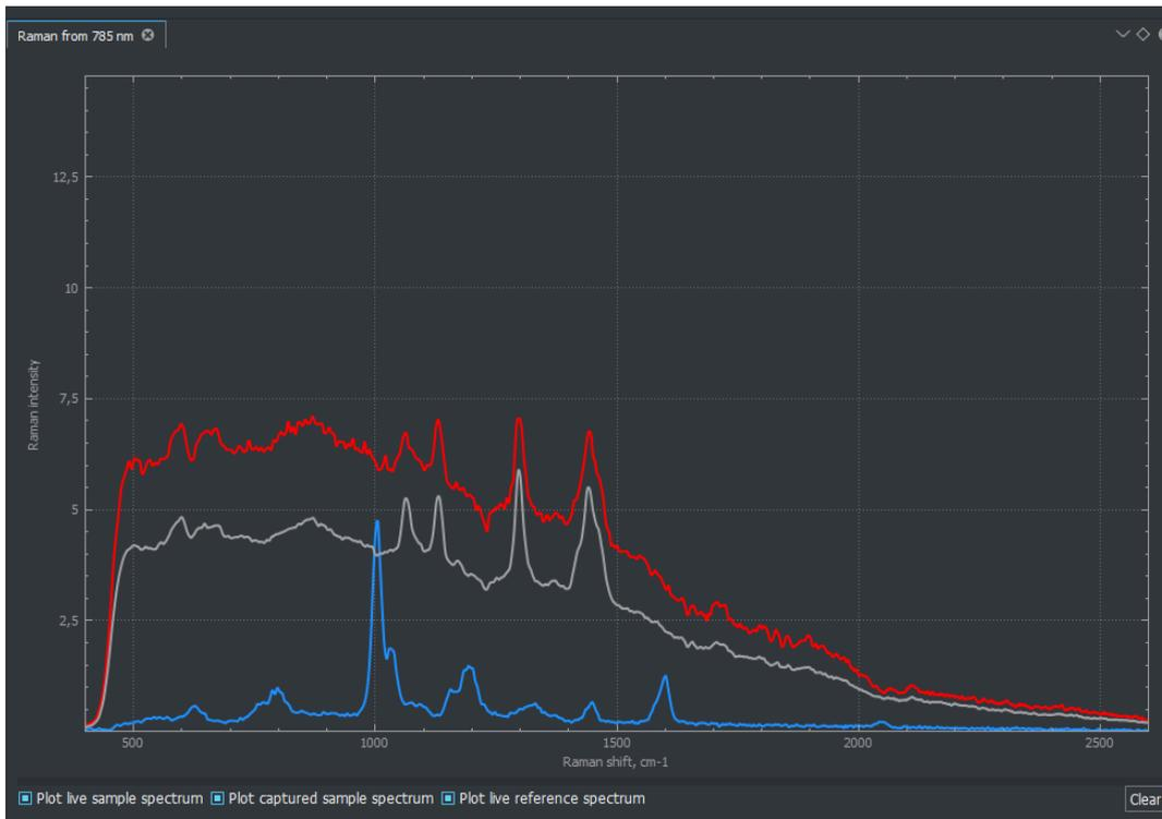
**Figure 17.** Illustration of spectrum capture which is done by averaging of fixed number of recorded spectra per time. Grey curve illustrates spectrum capture. Bottom menu allows to enable/disable showing necessary spectra.
