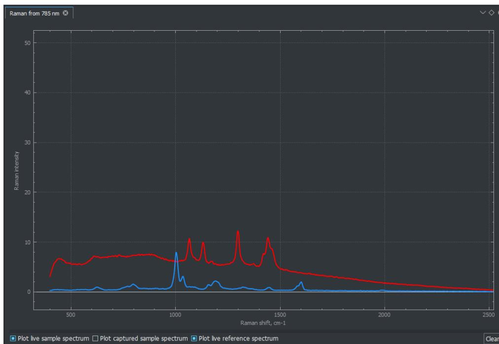
**Figure 11.** Different live spectra. Red curve corresponds to live sample spectrum, blue spectrum is polystyrene reference.
