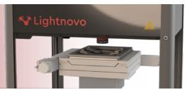
RG Raman microscope provides diffraction limited spatial resolution, extremely high throughput and additionally equipped with transmitted visible light microscopy on a separate camera sensor. RG Raman microscope can be used in upright microscopy and inverted microscopy configurations. All what is need for switching between modes – flip the device from top to bottom.
