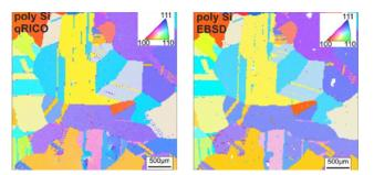
Fig. I. (A) orientation map of polycrystalline Si solar cell obtained by qRICO, (B) orientation map of polycrystalline Si solar cell obtained by electron microscope EBSD of the same area as shown on Fig. IA. The colors refer to the orientations as defined by the inverse pole figure (top right).
