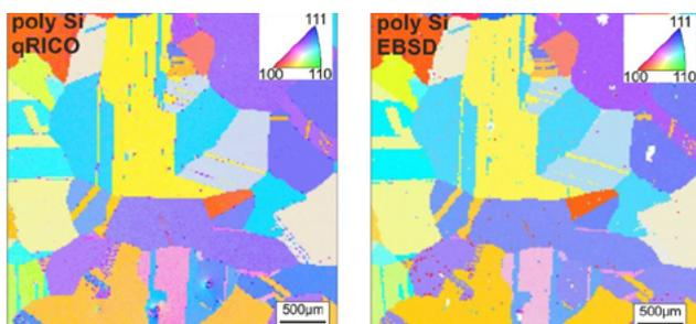
*Fig. 1. (A) orientation map of polycrystalline Si solar cell obtained by qRICO, (B) orientation map of polycrystalline Si solar cell obtained by electron microscope EBSD of the same area as shown on Fig. 1A. The colors refer to the orientations as defined by the inverse pole figure (top right).*
