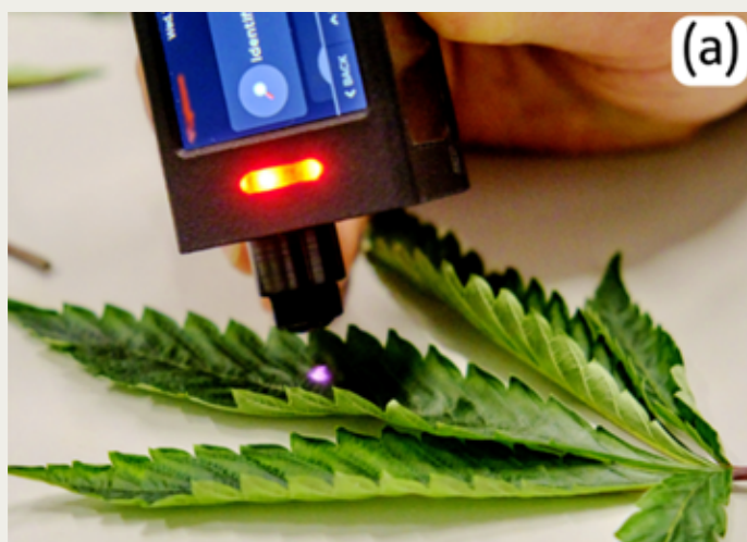
Figure 3. Measuring the spectrum from the adaxial (upper) surface of a cannabis leaf using the hand-held Raman spectrometer in (a) distant mode and (b) contact mode.
