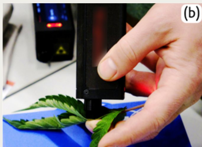
Figure 3. Measuring the spectrum from the adaxial (upper) surface of a cannabis leaf using the hand-held Raman spectrometer in (a) distant mode and (b) contact mode.
