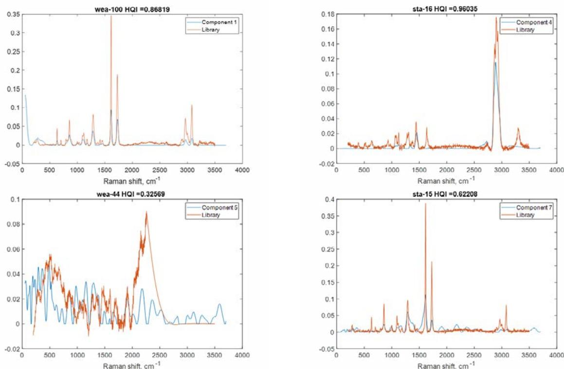
**Figure 7. Comparison of the Raman spectra for MCR-ALS components  $r = 1, 4, 5, 7$  with their best matches from database library [5].**
