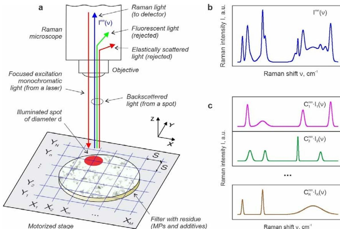
**Figure 1. 2D Raman mapping:**
