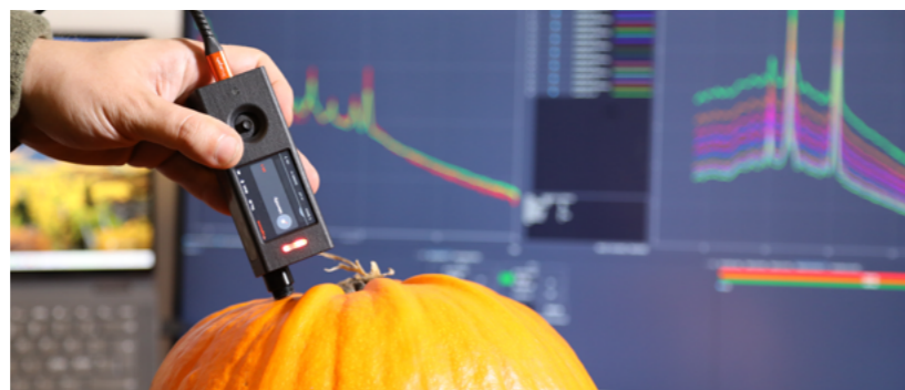
Figure 2. Measurements of pumpkin skin with miniRaman equipped with the contact probe.
