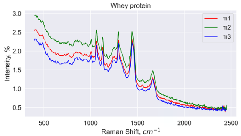
Figure 4. Raman spectra of whey protein sample measured through the plastic bag at different spots
