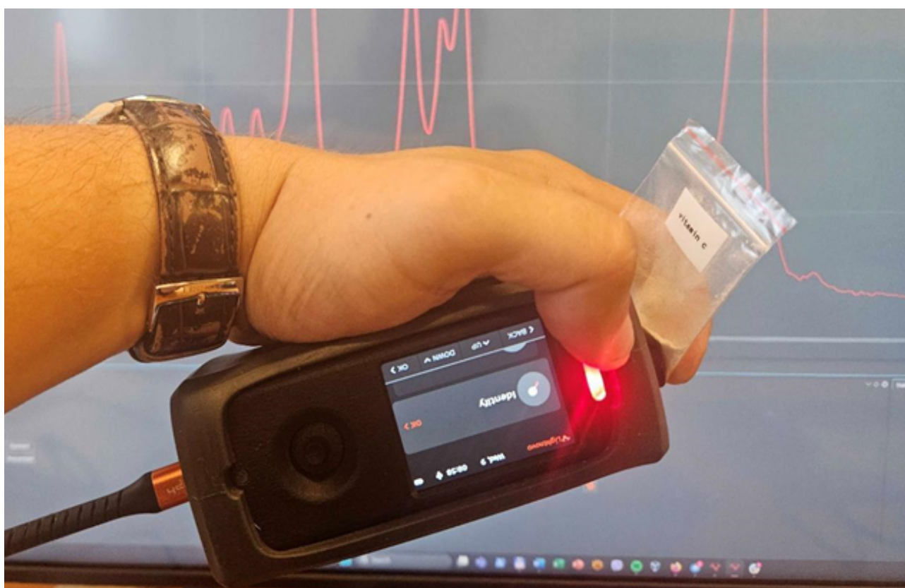
Figure 2. Measurement with Lightnovo miniRaman spectrometer: measurement of the vitamin C sample through a plastic bag with miniRaman spectrometer equipped with the contact probe. Live Raman spectrum of vitamin C in Miraspec software is displayed in the background.
