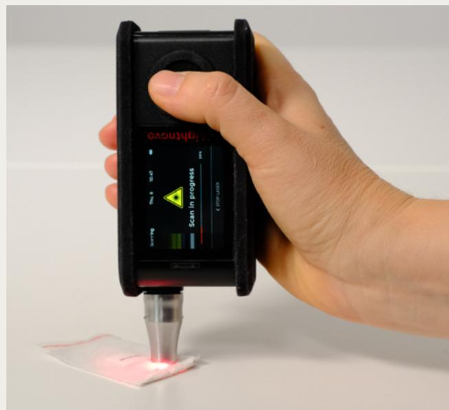
Figure 5. Lightnovo miniRaman 785 nm spectrometer.
