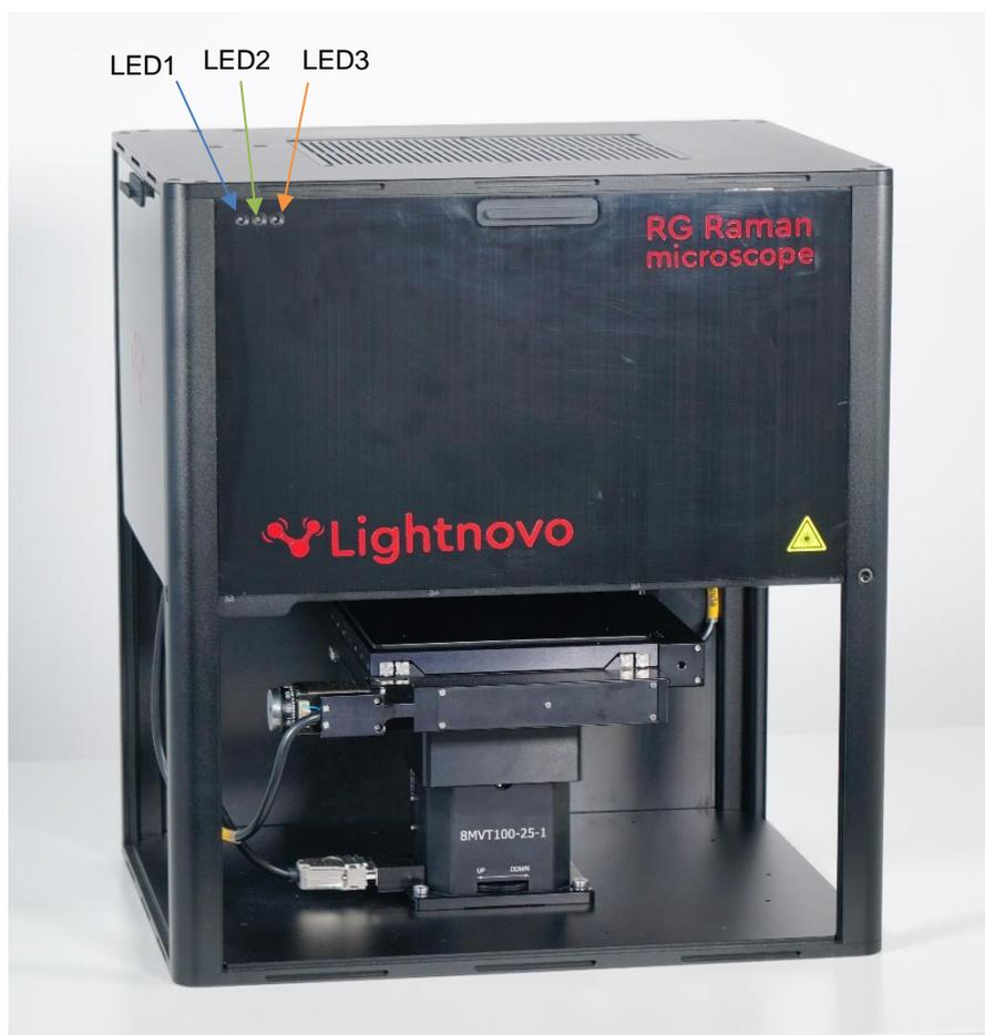
**Figure 5.** LED indicators of miniRaman microscope.
