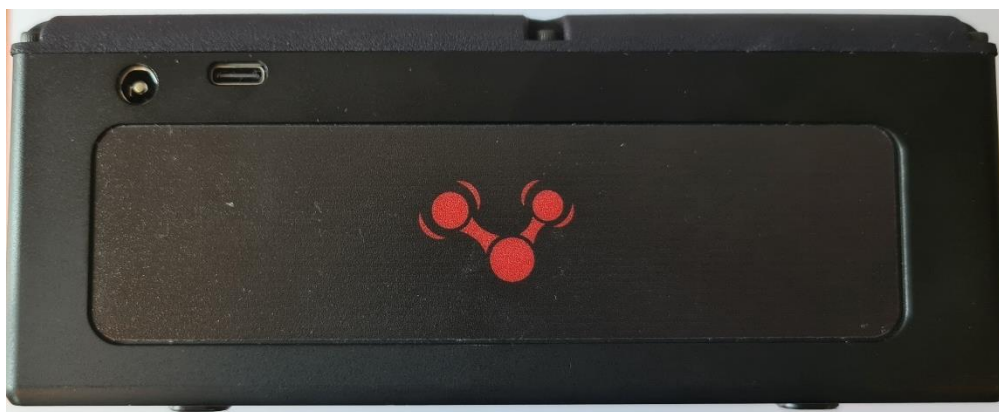
Figure 1. Side panel – overview of USB C and power supply connector sockets.
